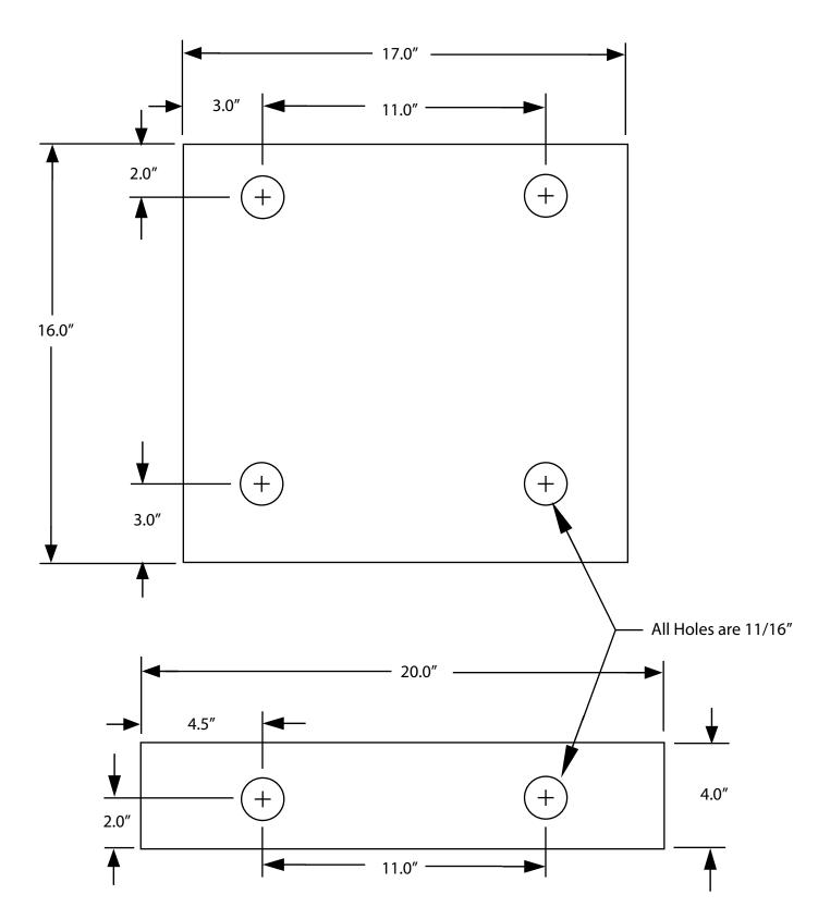
Holes in 4x20'' plate must line up with holes in 16x17'' plates so that bolts may pass all the way through them.
